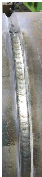
Pipe welding(3G) (170A/27V)
